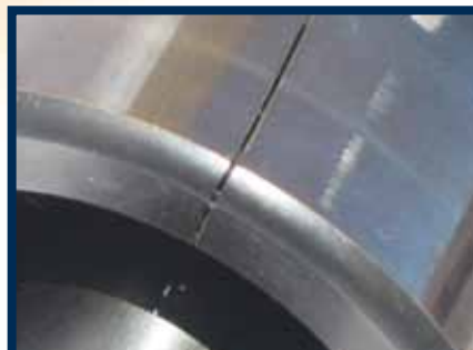
Roller Body Cracks or Shatters
