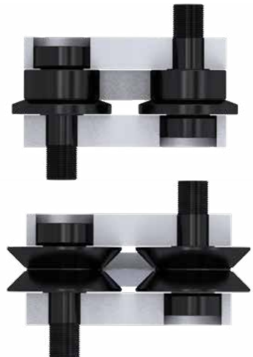
INCORRECT MOUNTING ALIGNMENT
